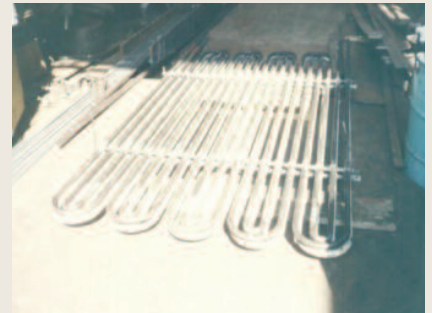
Fabrication of heating coils
