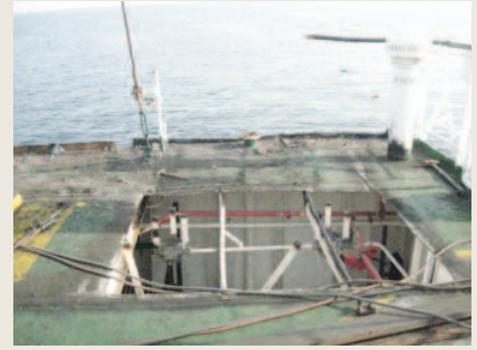
Side shell and deck collision damage on a bunker vessel (mid ship to the aft)
