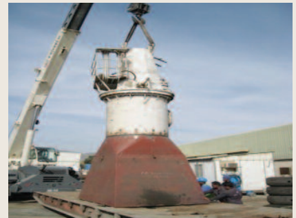
Fabrication of foundation for a mid ship crane
