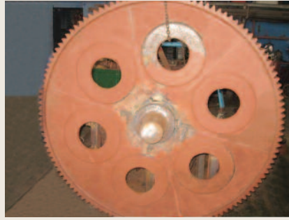
Repair of anchor winch gear
