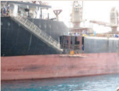
Repair of side shell collision damage at Fujairah Anchorage
