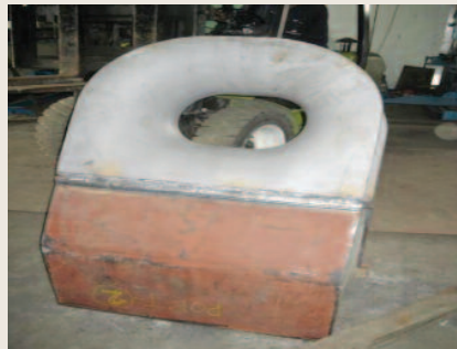
Fabrication of foundation for panama chock
