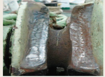
Build up welding of wildcut in situ
