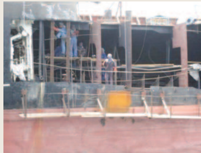
Repair of side shell collision damage at Fujairah Anchorage
