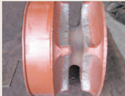
Build up welding on wildcut
