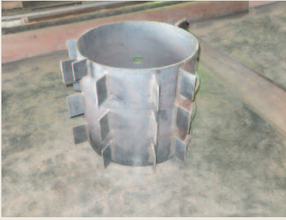
Fabrication of S/S cone burner for boiler
