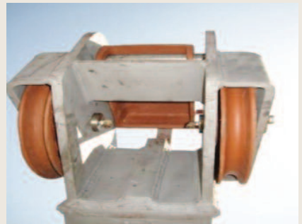
Renewal of crane boom sheaves
