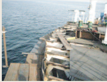
Side shell and deck collision damage on a bunker vessel (mid ship to the aft)
