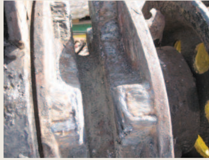
Build up welding of wildcut in situ
