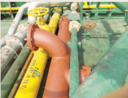
Renewal of diesel line on a bunker vessel
